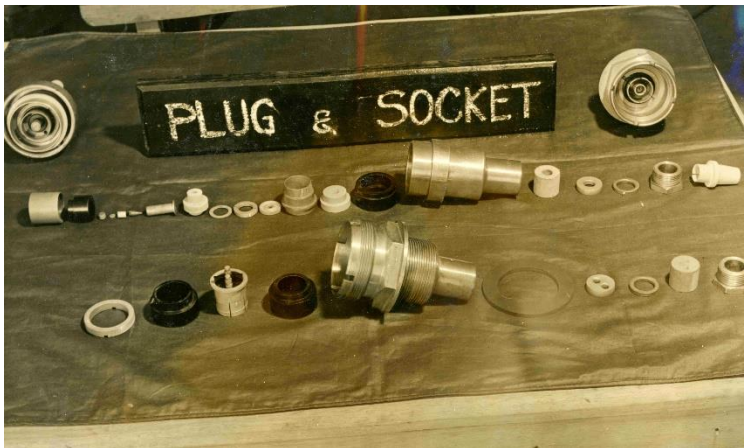
Fig 41: Parts of underwater plugs and sockets used on mines
