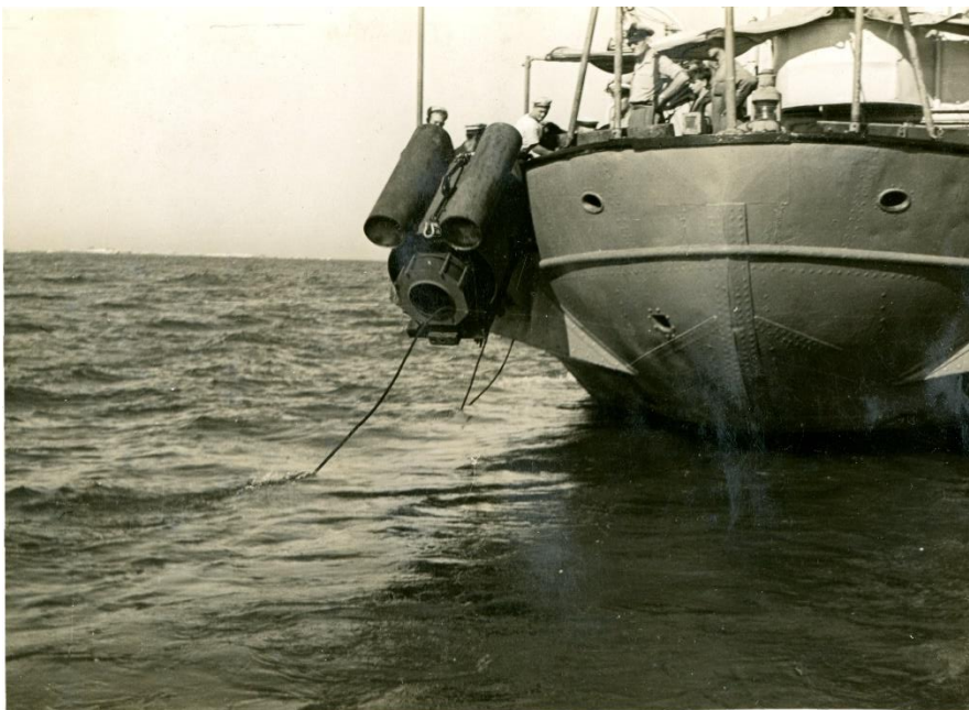
Fig 20: Mine falling
