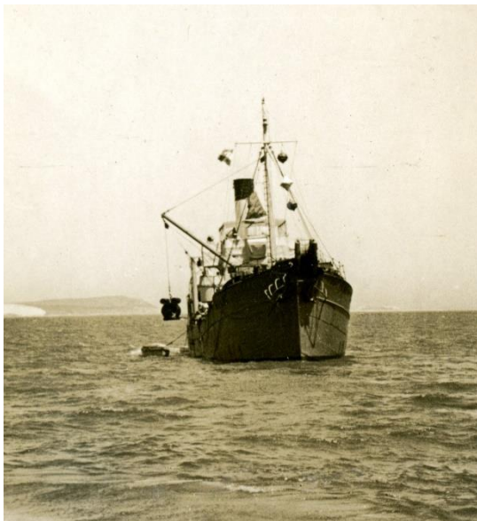
Fig 33: Mine suspended from Spindrift's derrick
