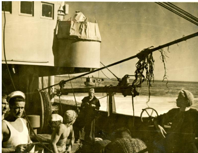
Fig 38: Tail cable being pulled in over head sheave
