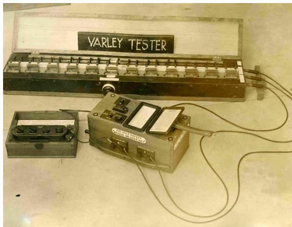
Fig 54: Varley tester for instruction in finding the position of earth faults on cables
