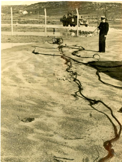
Fig 30: Recovered tail showing surf damage
