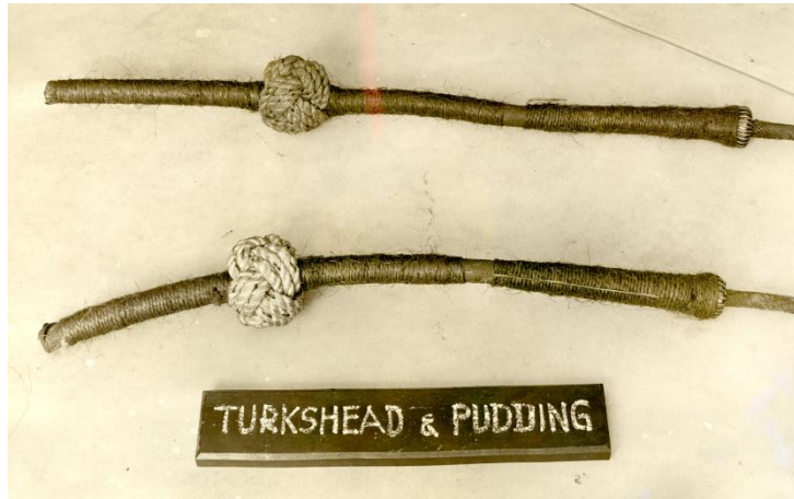
Fig 3: Locating the Turks heads and clamping puddings on electrical cables
