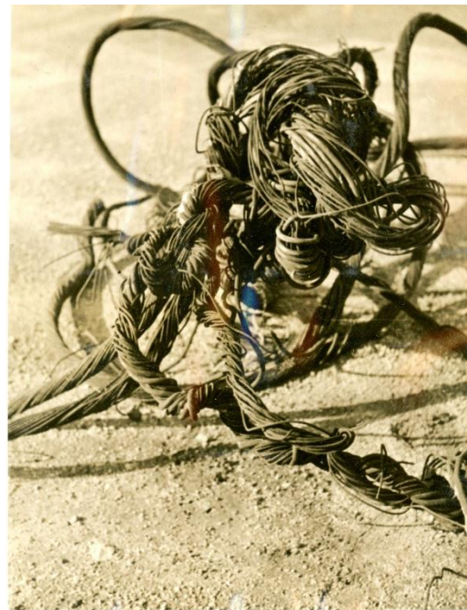
Fig 31: Close-up of surf damaged cable
