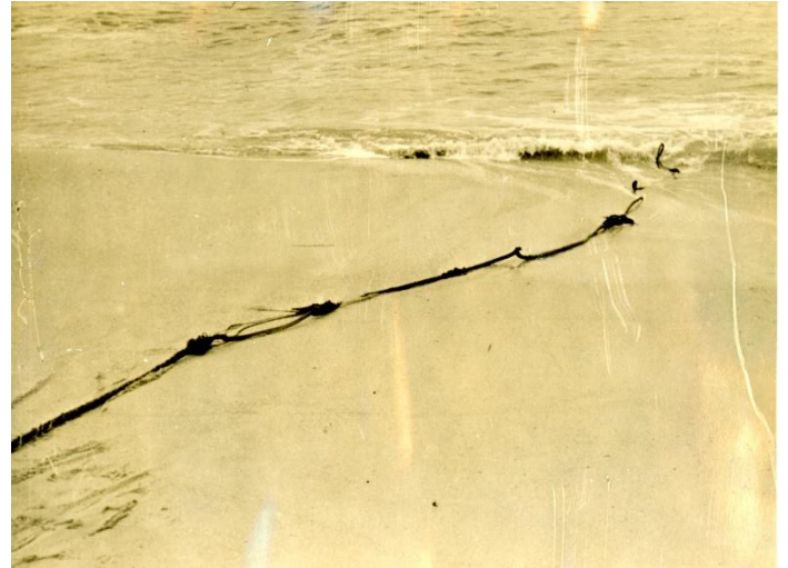
Fig 29: Tail cable damaged by beach surf
