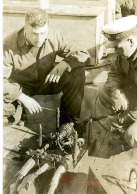
Fig 43: The main junction box opened on deck for inspection
